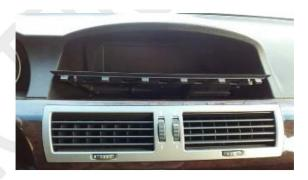
**3.** Proceed to the removal of the central part of the ventilation grille. Remove the screws ① with the T20 Torx-type screwdriver. Press out the central ventilation grill ② from the inside in the direction indicated by the arrow. Use a thin flat screwdriver to press the metal plate on top of the grill through the gap formed above, not allowing the metal plate to get stuck or break off from the grill body
