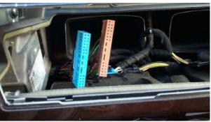
**6.** Release the IHKA ECU connector from the casing. Then pull off the fabric insulation of the connector for about 5 centimeters to free some space in order to be able to connect wire couplers to the wires of the connector.
