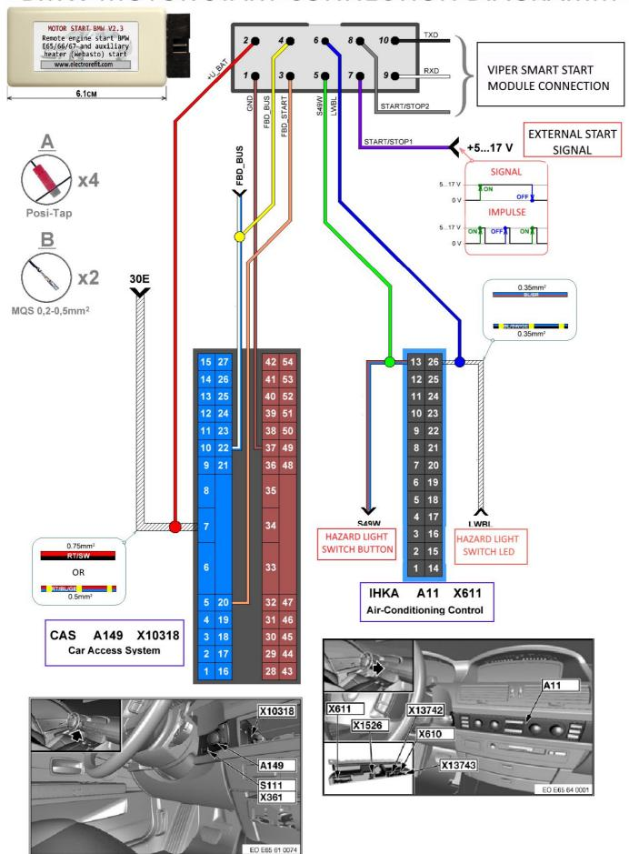
**8.** Find appropriate wires from the remote start module connector and connect them according to this diagram. I recommend installing POSI TAPS connectors further away from cases, so you can close it easily. Just move down factory isolation tape for some extra space. You need to insert 2 contacts female pins and tap 4 wires into existing wires. Please make sure you follow this diagram.
