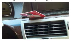
**2.** Then you need to grab the cover  $\bigcirc$  from the inside through the holes  $\bigcirc$  and by moving along the decorative strip, gradually release it from the clips by moving it upwards.
