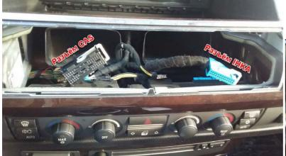
**5.** Release the 2-piece CAS ECU connector from the casing.
